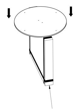
Step 2: Do not fully tighten the bolts.
